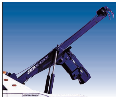
Fabricated Hi-Tensile Steel Recovery Boom
