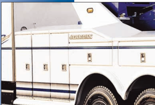
Lightweight, Corrosion-Proof, Bonded composite & Aluminum Body
